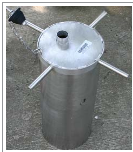
Figure 2. Stainless steel corer 20 cm diameter used to collect seagrass samples.
